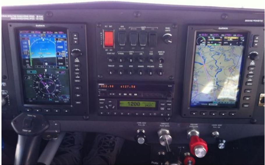
To the left you see our 'in flight' view. The left display looks like an F15 with synthetic vision. The right screen shows engine detail and a moving map. Between them is circuitry, comm-radio and Mode C. No round dials.
